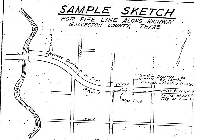
NOTE: Give Chained Distance from Line to End of Bridge, End of Culverts with Headwalls, Center-Line of Underpass, or Center-Line of Inter-secting Highways.
